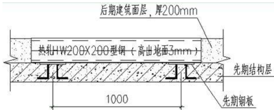
Figure 25 Schematic of indoor GIS foundation section (generic equipment number 1GIS-2000/40 )
