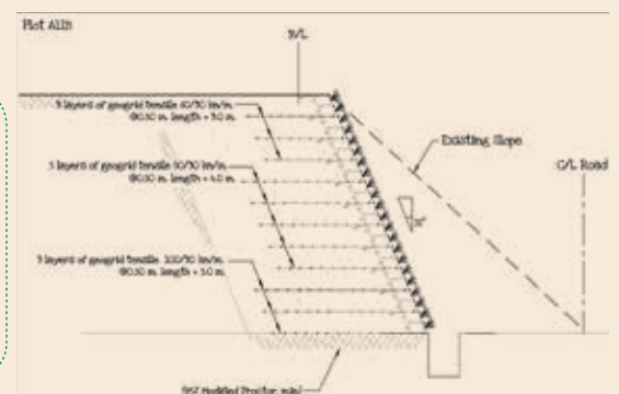
Steep Slope Reinforcement using soil bag reinforcement and Geogrids facing Plot A11B, Hemaraj RIL.
